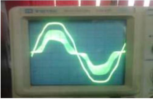
Fig. 9. Input current & voltage waveforms with PFC
