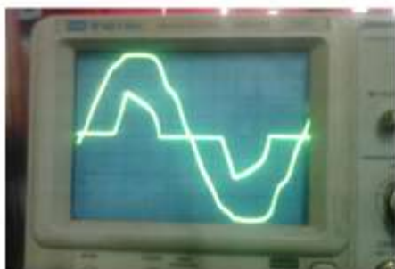
Fig. 7. Input current & voltage waveforms without PFC.
